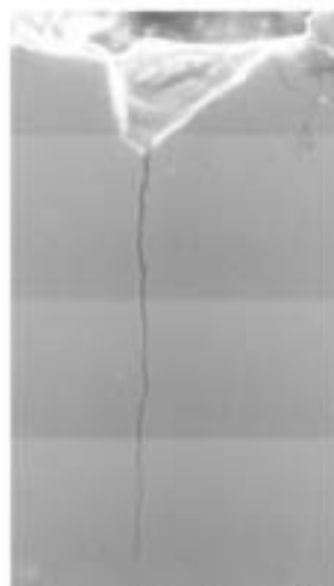
図3 被覆処理材の疲労き裂発生 \sigma = 140 MPa, N_f = 2.8 \times 10^5
